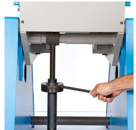
Inclination adjustment (hydraulic on 45 and 80T)
