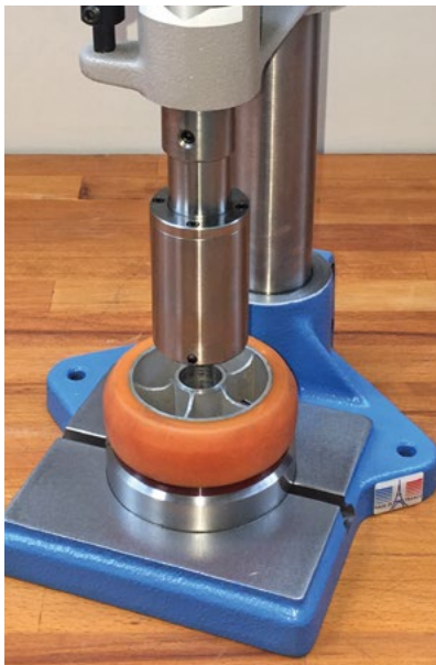
▶ 4HR with bearing mounting tooling
