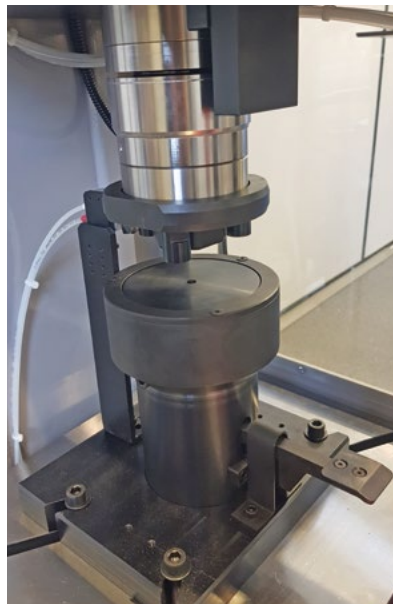
▶ 13T HYDRO with deformation tooling
