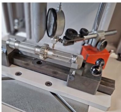
▶ 6TLP with shaft straightening tool
